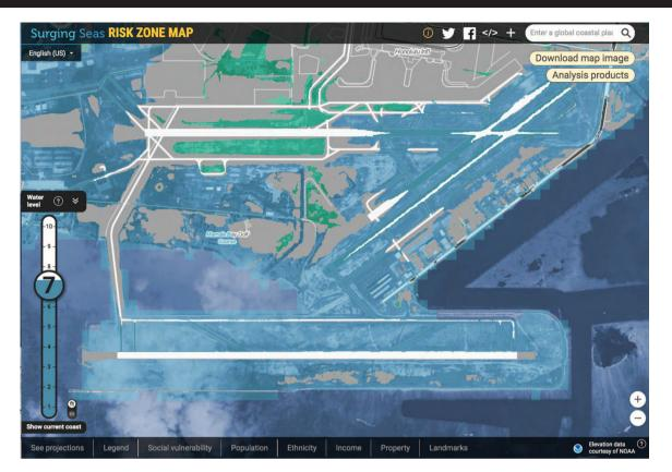
Figure 13. Honolulu International Airport with 7 ft (2.1 m) of sea-level rise above MHHW. Blue areas would be flooded. Green areas are below 7 ft (2.1 m) but are protected by some barrier. (Source: Climate Central Surging Seas.)
