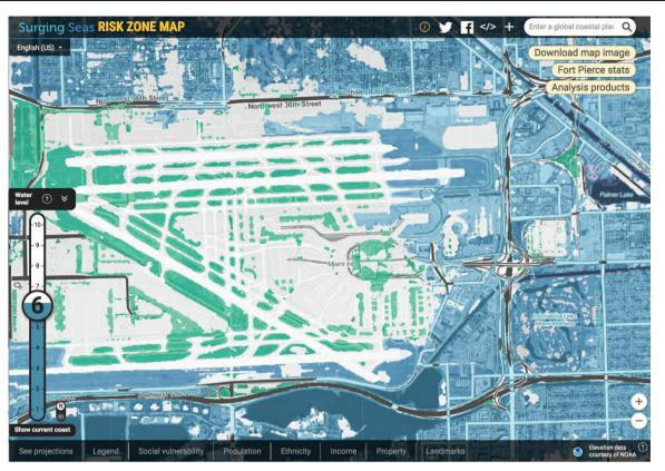
Figure 11. Miami International Airport with 6 ft (1.8 m) of storm surge or sea-level rise above MHHW. Blue areas would be flooded. Green areas are below 6 ft (1.8 m) but are protected by some barrier. (Source: Climate Central Surging Seas.)
