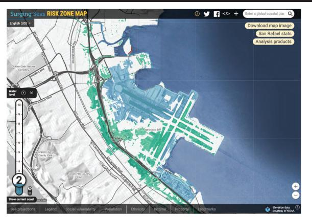
Figure 2. San Francisco International Airport with 2 ft (0.6 m) of sea-level rise above MHHW. Blue areas would be flooded; green areas are less than 2 ft (0.6 m) above MHHW but are separated from San Francisco Bay by some barrier. (Source: Climate Central Surging Seas.)
