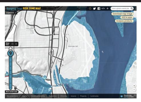
Figure 15. Washington National Airport with 9 ft (2.7 m) of storm surge or sea-level rise above MHHW. Blue areas would be flooded. (Source: Climate Central Surging Seas.)
