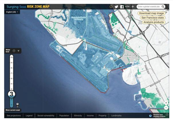
Figure 9. Oakland International Airport with 3 ft (0.9 m) of storm surge or sea-level rise above MHHW. Blue areas would be flooded. (Source: Climate Central Surging Seas.)
